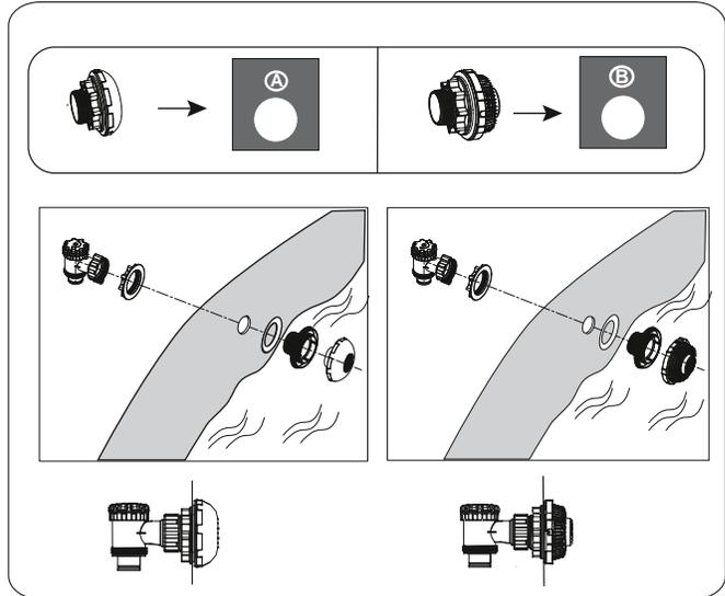
**NOTE:** If you want to connect other pool cleaning kits to the pool through the connection valve, use a Phillips screwdriver to disassemble the Debris Screen from the Connector.
